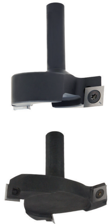
FIGURE 2: These spoilboard surfacing cutters are used for surfacing MDF, particleboard and balsa core where “flow through” or “high flow” cutting is employed using large capacity vacuum pumps.
